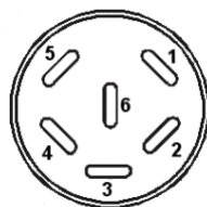
Figure 19: Pin allocation of socket (10) for option analog output
