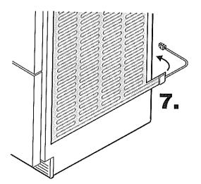
7. Bend the lower tongue of the heating blanket around the corner and adhere to the back of the appliance.
