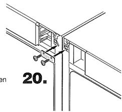
20. Attach the connecting plate and fasten with the screws of step 19.
