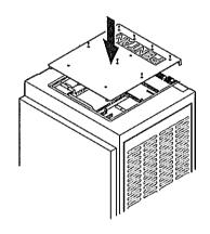
**14.** Position the top cover and screw into place.
