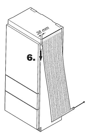
**6.** Adhere the heating blanket on the top of the left unit. Upper edge of blanket flush with the appliance top. Front edge of blanket 38 mm from the appliance housing backwards.
