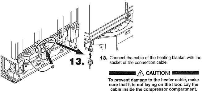
Do not lay the cable inside the evaporation tray of the compressor!
