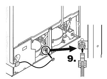
**9.** Connect the cable of the heating blanekt with the socket in the compressor compartment.
