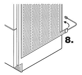
**8.** Bend the lower tongue of the heating blanekt around the corner and adhere to the back of the appliance.
