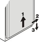
**8.** Tilt door inwards from the left **1**. Secure hinge pin with screw **2**.
